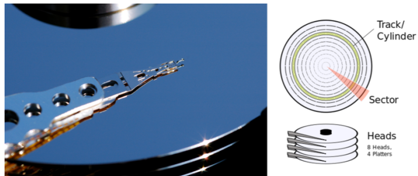
The functioning and parts of a hard disk drive. Source: Wikipedia.
